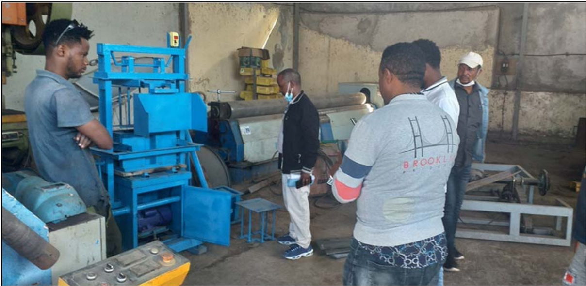
Testing the concrete block making machine
